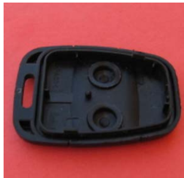
Top cover of remote with fitted from outside replacement buttons. (Internal view of the top cover)
