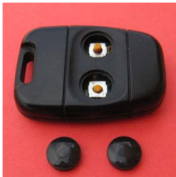
Nissan remote after removal of an old rubber insert with embedded buttons
